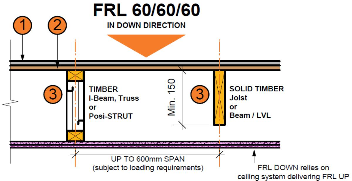
Figure 1 Timber frame floor/ceiling system with 1 × 19 mm INEX>FLOOR19 on top of plywood or particleboard Flooring
