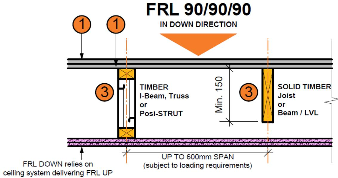
Figure 3 Timber frame floor/ceiling system with 2 × 19 mm INEX>FLOOR19
