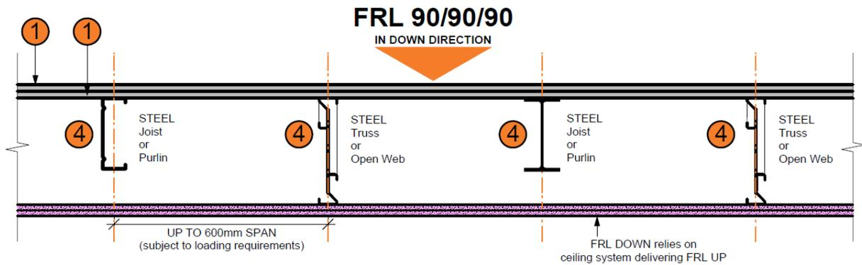
Figure 4 Steel frame floor/ceiling System with 2 × 19 mm INEX>FLOOR19
