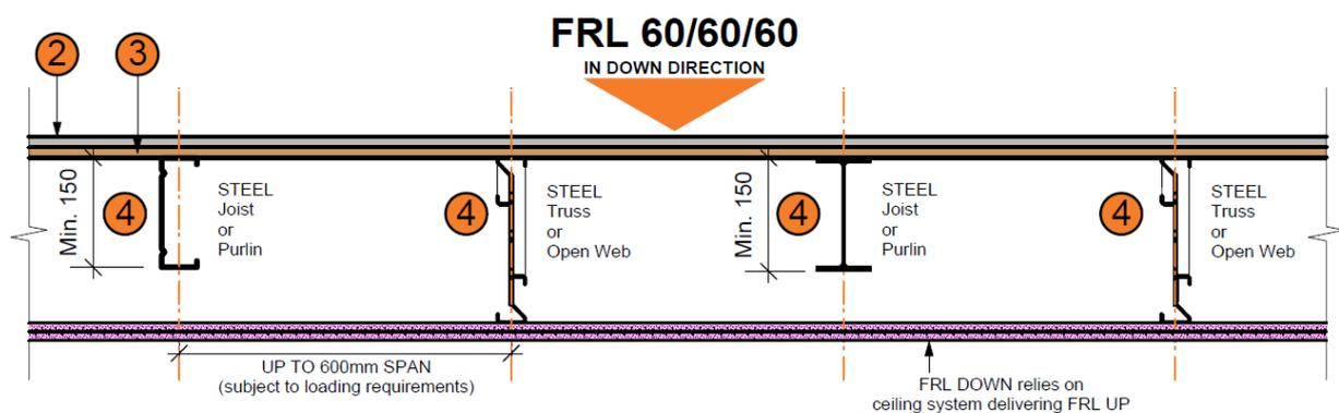
Figure 2 Steel frame floor/ceiling system with 1 × 19 mm INEX>FLOOR19
